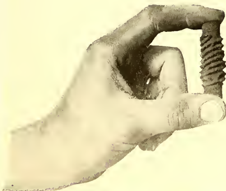
A Bound Brook Mold. The graphite cannot be forced out under pressure.
